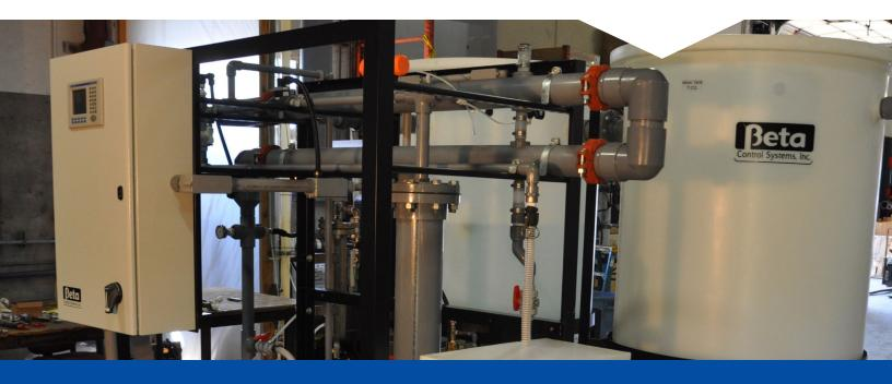
Recycle dirty flux solution using our Oxyfilter's crossflow microfiltration membranes.
