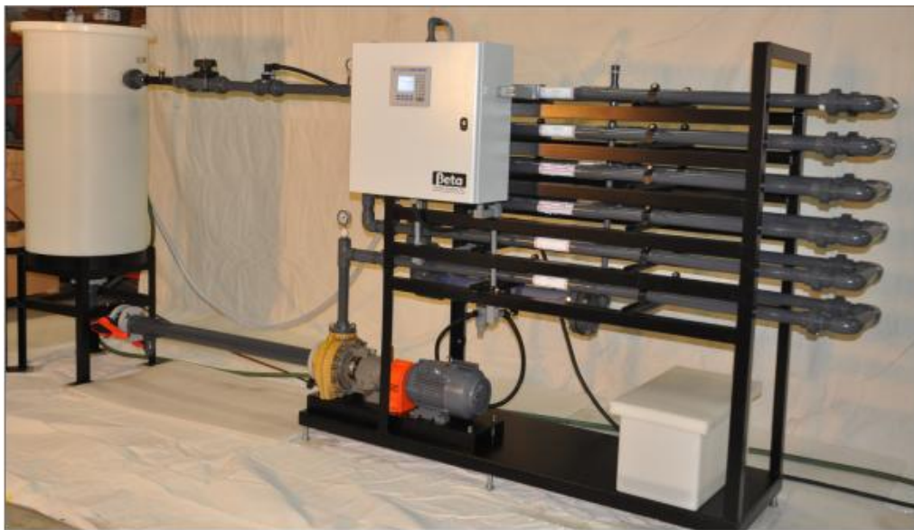
Figure 4 - Crossflow Microfiltration Membranes on the Oxyfilter System
